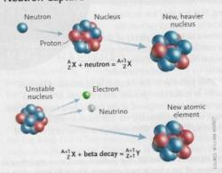
PARTICLE PINBALL When an atomic nucleus captures an extra neutron, it becomes a heavier isotope of the same atom. (Here Z is the number of protons and A, the atomic number, is the combined total of protons and neutrons.) If the new isotope is unstable, one of its neutrons may decay into a proton by emitting an electron and an antineutrino, converting the atom into the next element in the periodic table.
